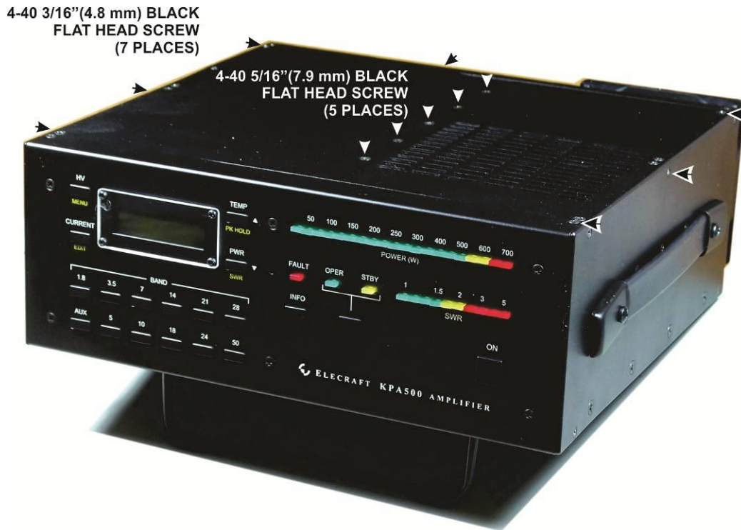
Figure 64. Top Cover Installation.
