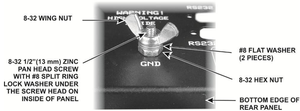
Figure 21. Installing the Rear Panel Ground Lug.
