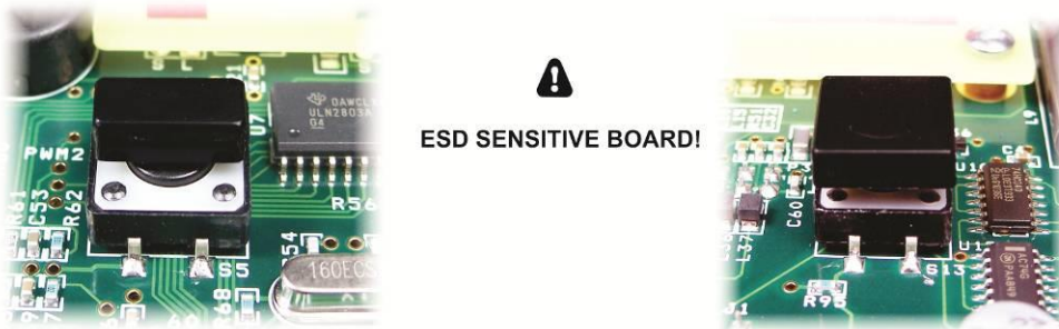
Figure 57. Installing Key Caps on Front Panel Board.
